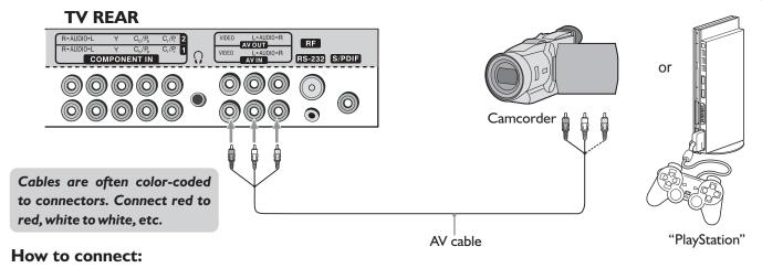
Connect the Audio/Video cables between the Audio (L/R)/Video jacks on the unit and camcorder.
